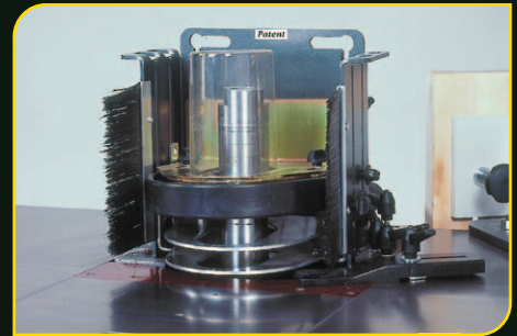
Safety protection for round profiles Profilschutzhaube
